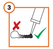
When using Shufit Glue, express a small amount of glue until it is dark grey before using.
