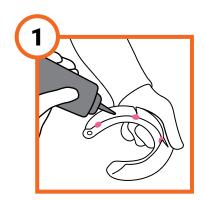
Put four medium beads of Shufix on the inside base of the shoe and cuff.
