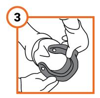
Holding back the side cuffs, aligning it with the frog and adjust to the correct position.
