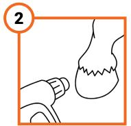
Make sure the hooves are dry. Most glue failure is due to dirt or moisture in the hoof.
